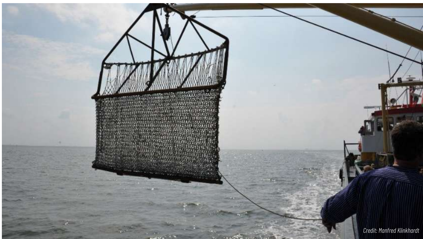
When collecting oysters, scallops and mussels, dredges are commonly used, which are towed close to the seabed.
