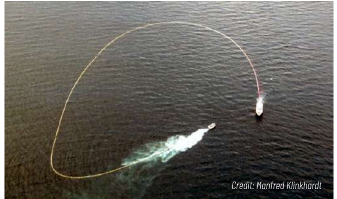
The use of purse seines requires the precise location of rewarding schools of fish, which are then encircled with the surrounding net.
